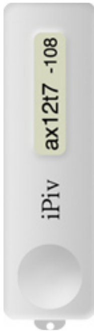
The image shows an iPiv prototype. Please note, on the display, the 108 seconds before the expiration of the current electronic identity.
